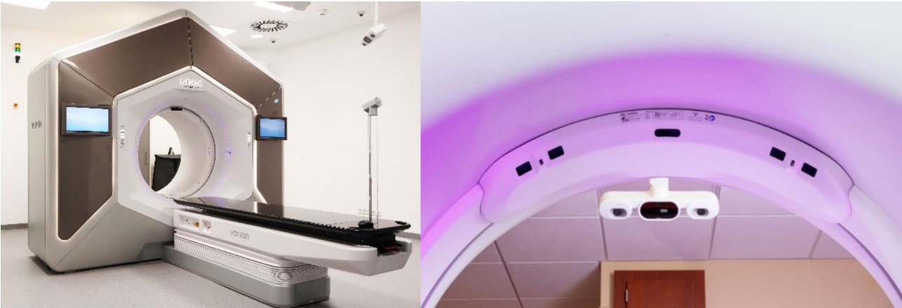
Fig. 1 Left panel: Mannheim Ethos LINAC and outer 3D cameras from AlignRT; Right panel: Rear view of AlignRT inBore miniature cameras (VisionRT.com)
